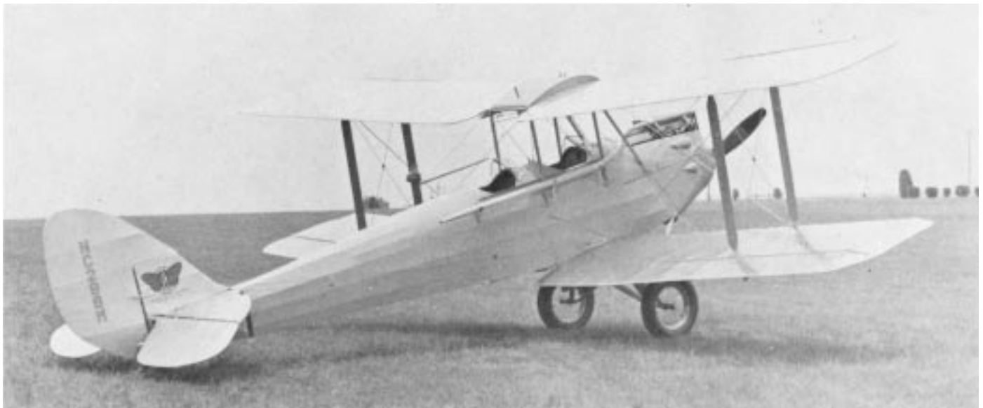
Gipsy Moth NC298M was like those flown in tour. Picture shows center-section fuel tank, wooden interplane struts, long exhaust pipe and typical DH rudder.
