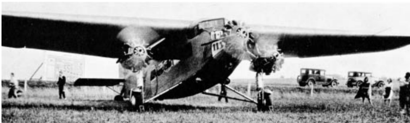
George Chapline running up the Wright Aero Ford, at Cedar Rapids. Note long exhaust pipes; big landing lights on belly. Billboard in background advertises "Russell's Ice Cream." (Charles Scheetz)
