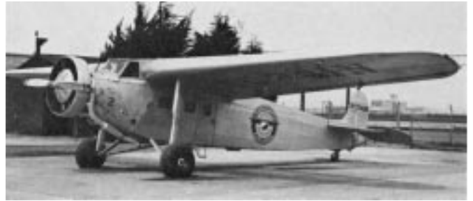
Fokker Super Universal, NC-341-N at Alameda, California, was similar to Goodyear ship which accompanied tour; has big doughnut tires sold and publicized by Goodyear as "Airwheels." (Mrs. Carl Bigelow)
