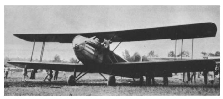
The Douglas C-1, Pathfinder and Official Press plane. Pilot and mechanic sat in cockpit just behind. Liberty motor; eight passengers rode in enclosed cabin. (Ford/Hudek)
